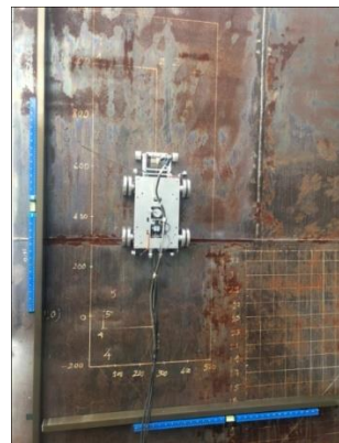
Figure 2.4: Positioning and installing the standard ruler in the two directions x, y
